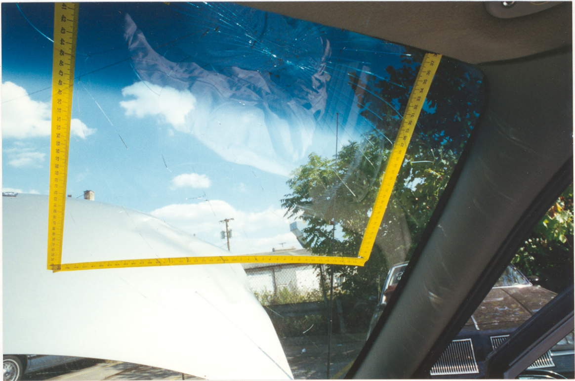
65. Overall view of the windshield fracture caused by the deploying passenger side air bag.
